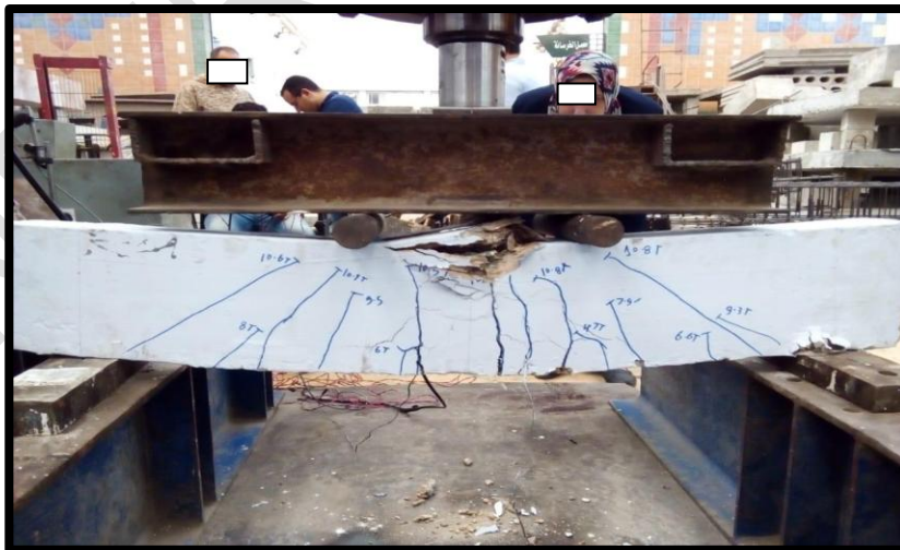
FIG. 7 Sample of cracks propagation and mode of failure
