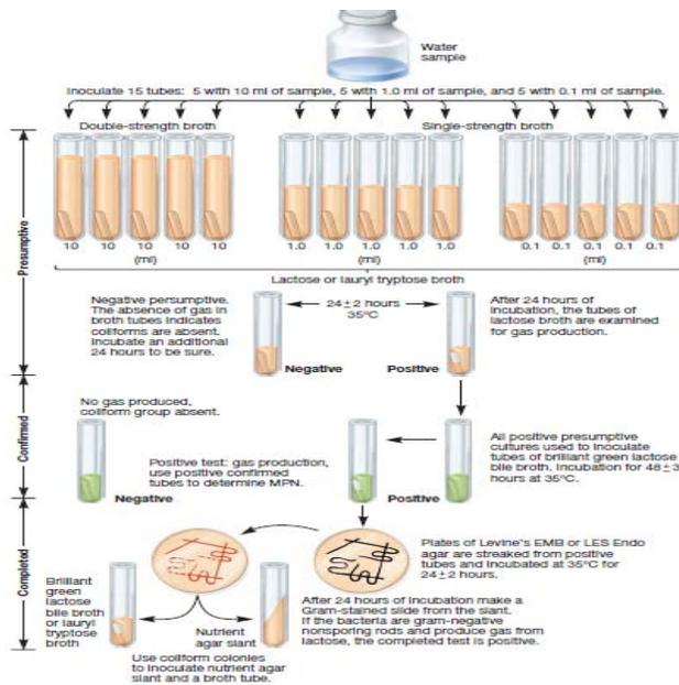
**Figure 1: Multiple Tube Fermentation Technique for Water Testing**
