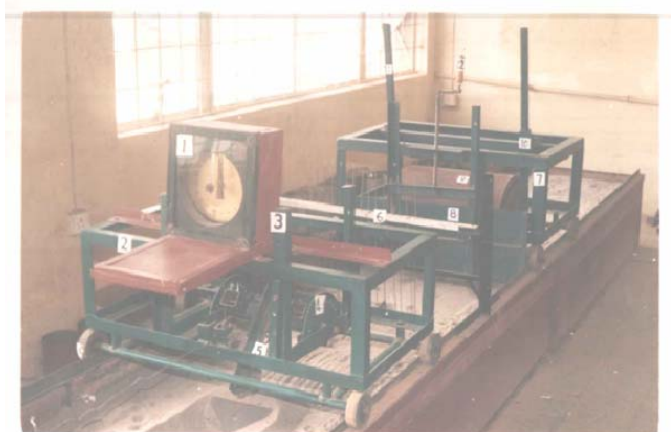
Figure 7. An indoor soil bin at FUTA (Manuwa and Ademosun, 2007)
