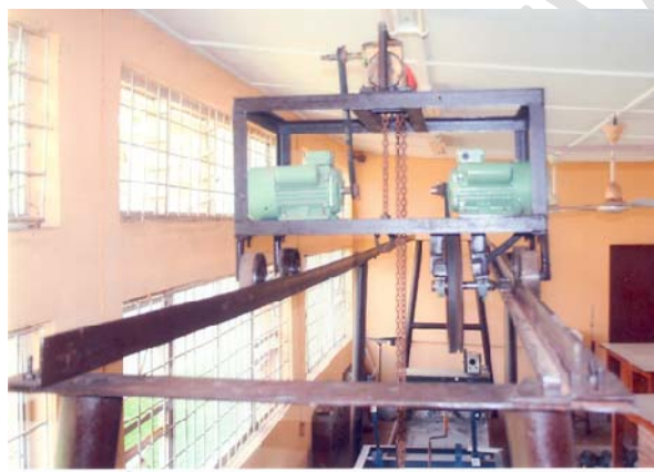
Figure 8. Indoor Soil bin (FUTA) with overhead gantry crane (Manuwa and Ajisafe, 2010)
