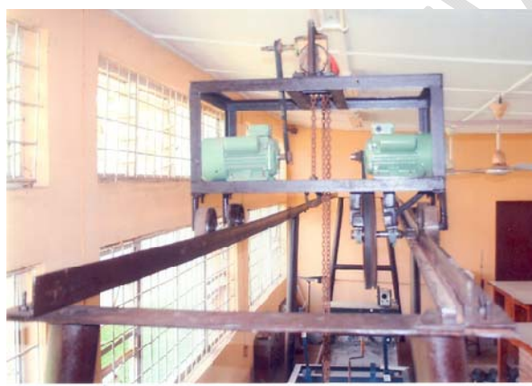
Figure 8. Indoor Soil bin (FUTA) with overhead gantry crane (Manuwa and Ajisafe, 2010)
